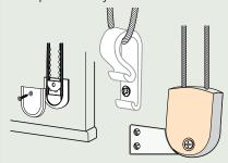
Chain-break connector or Safety tassel These will break apart when when undue pressure is applied to the
