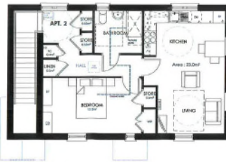
FIRST FLOOR PLAN TYPE F2 2P1B General Needs - 54.9m 2 Stair = GF - 5.2m 2 + FF - 7.3m 2 = 12.5 m 2
